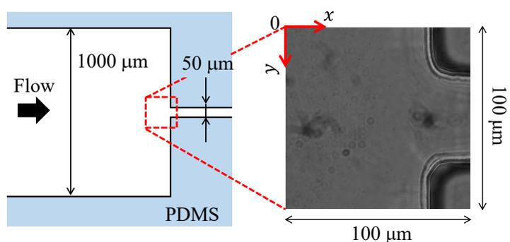
Fig. 2. Schematic of a sudden contraction microchannel and a transmission image of the measurement area of fluorescence imaging.
