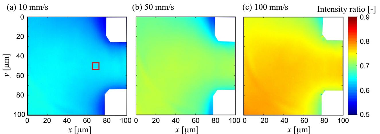
Fig. 5. Distributions of the intensity ratio of green (529 nm) to blue (494 nm) fluorescence measured at different flow rates. The cross-sectional average velocity in the contraction channel was (a) 10 mm/s, (b) 50 mm/s, and (c) 100 mm/s.
