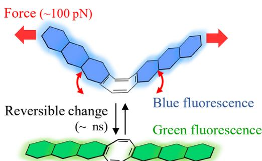
Fig. 1. Reversible change in molecular conformation and fluorescence color of FLAP in response to external force.
