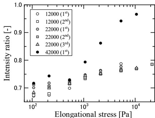
Fig. 4. Relationship between the measured fluorescence intensity ratio and the elongational stress estimated by simulation.
